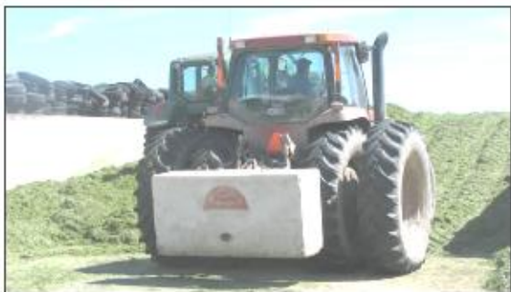
Figure 1: Concrete blocks and an extra tractor are effective ways to increase packing weight and silage density.
